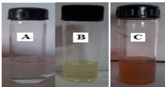
Figure 1 (A) silver nitrate solution (B) Citrus sinensis peel extract and (C) brownish orange color indicating the formation of silver nanoparticles.
